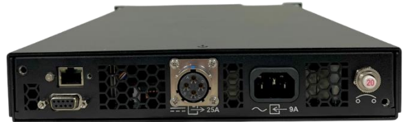
Rear Panel with AC IN, DC OUT, Communications, and SNMP Interfaces
