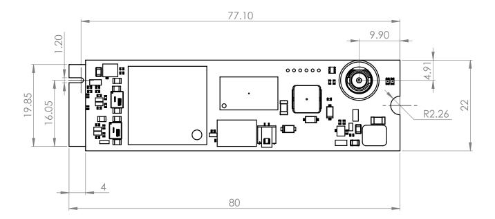
Dimensions are in millimeters.
