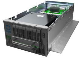
As the latest product in One Stop Systems' line of PCIe storage expansion, Centauri offers high-capacity storage in a compact chassis. Built as a modular storage expansion to the OSS 3U SDS, Centauri can store up to 256 TB in its 8-drive canister. These canisters allow for tool-less bulk or individual drive removal and can be hot-swapped for ease of use in fast-paced environments.
