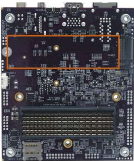
Bottom view of STEVIE showing the M.2 2280 socket (outlined).
