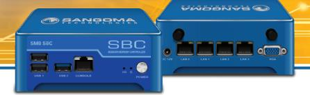
IP communications across multiple, sometimes untrusted, networks needs to be normalized, managed and secured. There is a need to guarantee interoperability of multiple devices, carriers and protocols in a transparent way to the user of the network. Session border controllers take care of the conversion between protocols, transcoding, threat prevention, resource limiting, and accounting at the edge of VoIP networks of enterprises and carriers alike.
