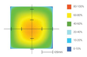
Optical measurement taken using CB0404-WHIIC
