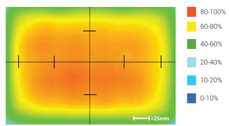
Optical measurement taken using BL-S100150-WHI
