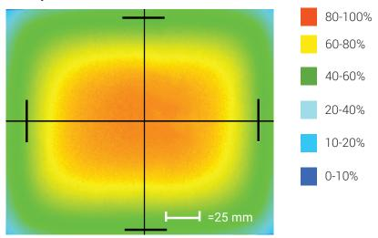
Optical measurement taken using BL-S050075-WHI
