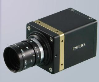
The IGV-B4020 is an advanced high-speed progressive scan, fully programmable CCD camera designed for imaging applications that require high frame rates, high quality images, and powerful features and flexibility. The camera has a small size, light weight, and is built around Kodak's KAI-11002 Interline transfer CCD image sensor with a 43.3 mm image diagonal. ICL-B4020 features CameraLink output. IGV-B4020 features GigE Vision output.
