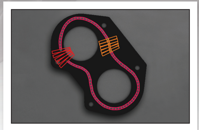
MIL Bead Inspection
