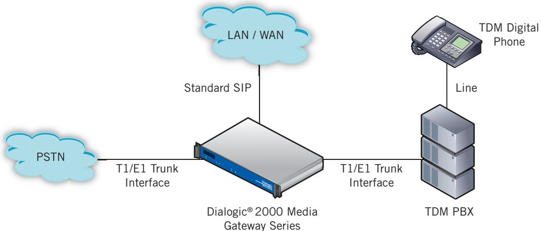
Figure 4. Access Gateway with Survivability Capabilities
