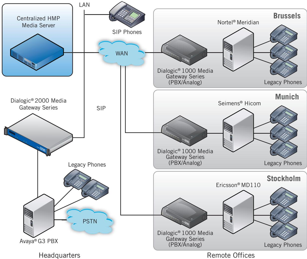
Figure 2. Converged IP Media Server Architecture
