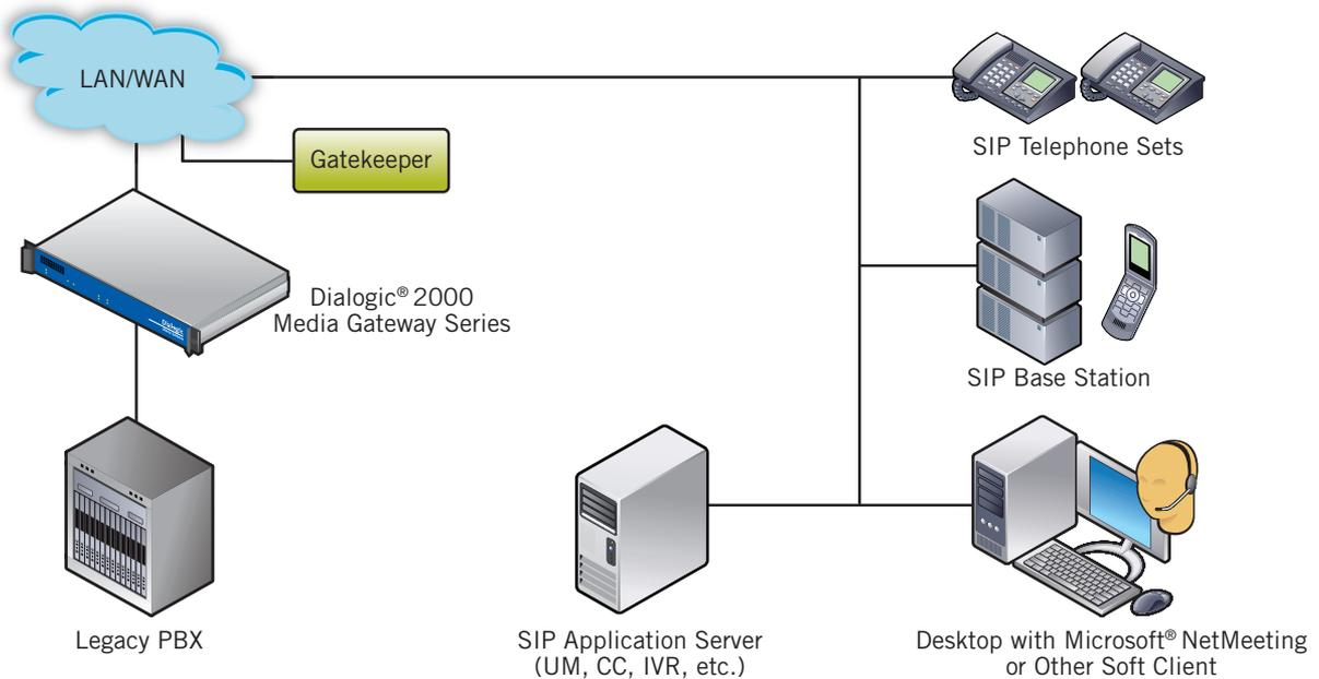
Figure 1. Bridge the Gap Between PSTN and IP End Points
